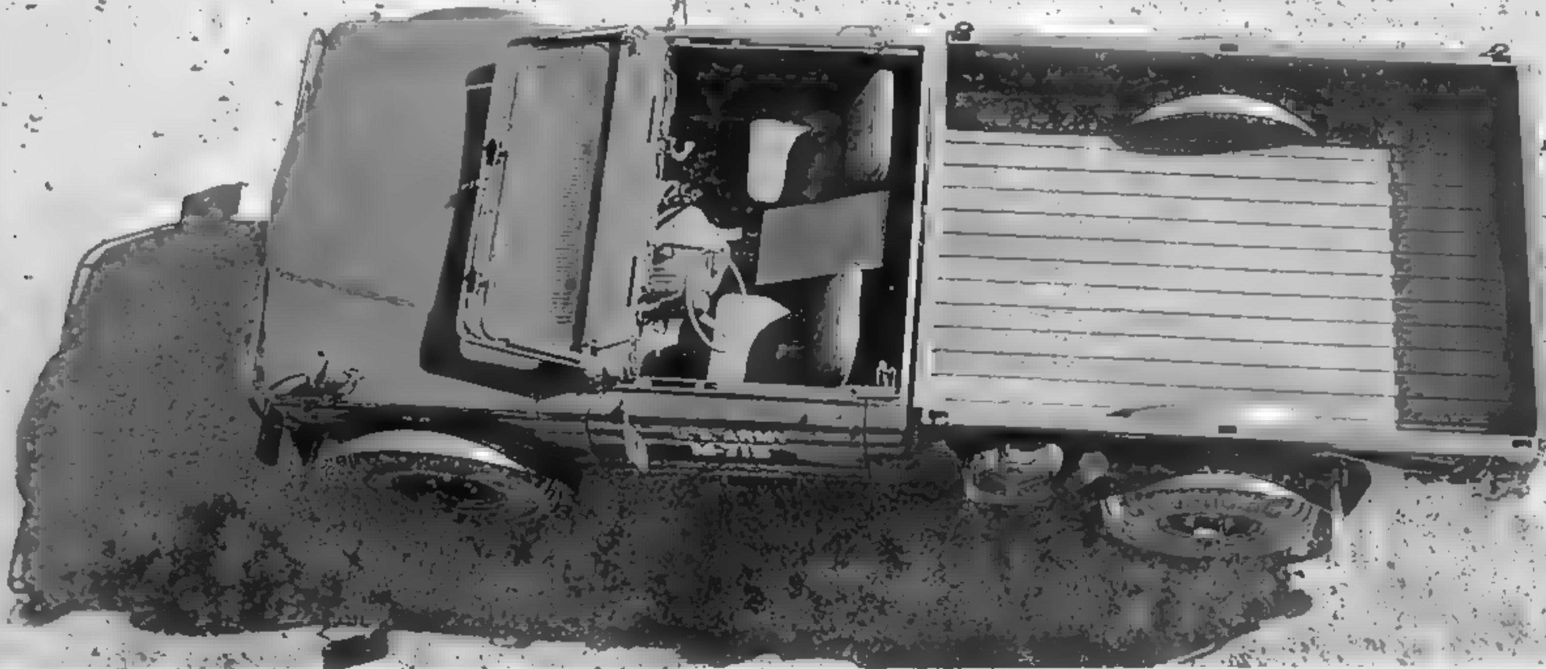
The XM715 is shown with all the canvas removed and the windshield folded down. The unusually shaped box between the seats is the truck's battery box. The fuel filler and spare fuel can be seen in the lower part of the photograph. (Photo courtesy the Patton Museum)
